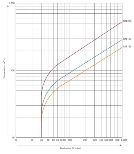
Druckverlust = pressure loss Volumenstrom = volume flow
